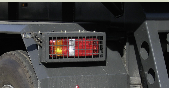
Protection grid for rear lights.
