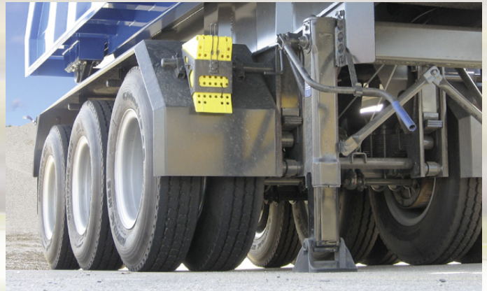
The continuous mudguard minimizes soiling and protects the tyres against falling bulk material during loading.
