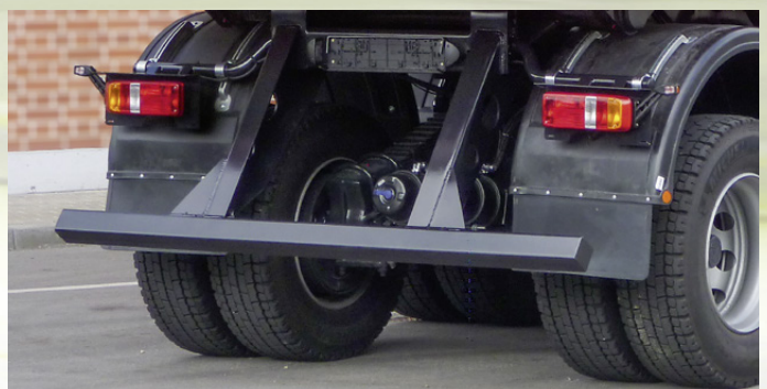
The tipping semi-trailer can be equipped with a rugged underderride guard that withstands considerable impacts.
