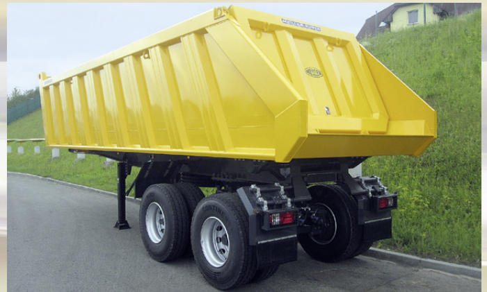
Interior tailgate. Ideal for finisher use: the 2-axle tipping semi-trailer.
