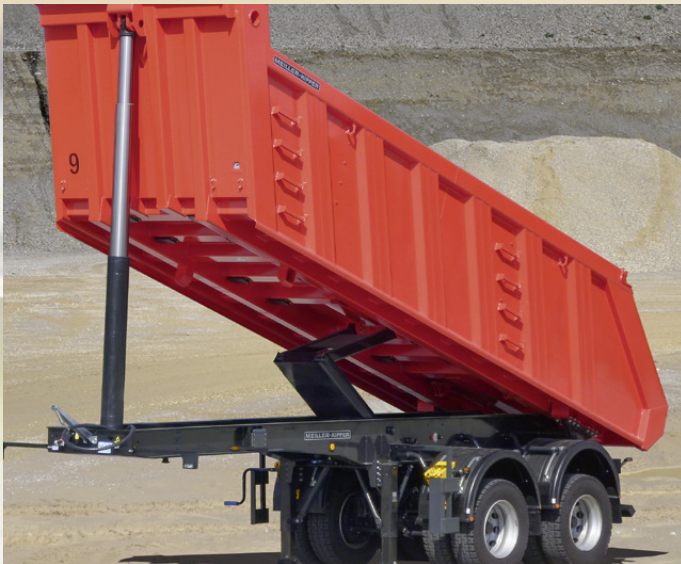
Interior tailgate. Ideal for finisher use: the 2-axle tipping semi-trailer.
