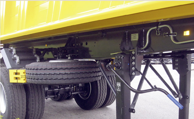
Bolted sparer wheel carrier for the spare wheel – optionally 1 or 2 wheels under the chassis frame of a 2-axle vehicle.
