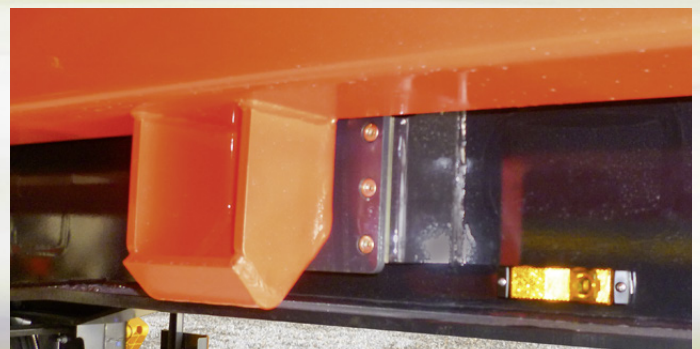
A sturdy tipper body guide centres the body after tipping.
