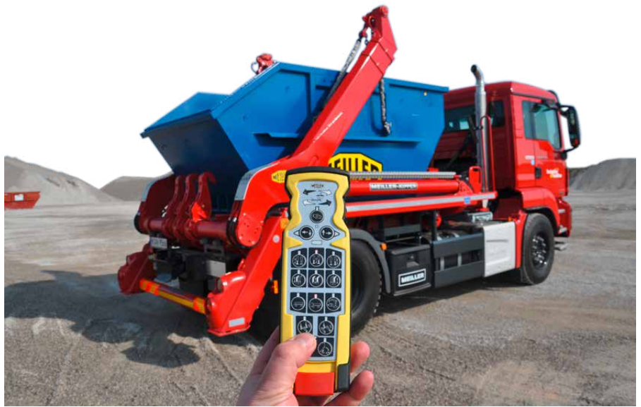
Always control your sequences fast and safely with the practical i.s.a.r.-control remote control, here the AK12-MT
