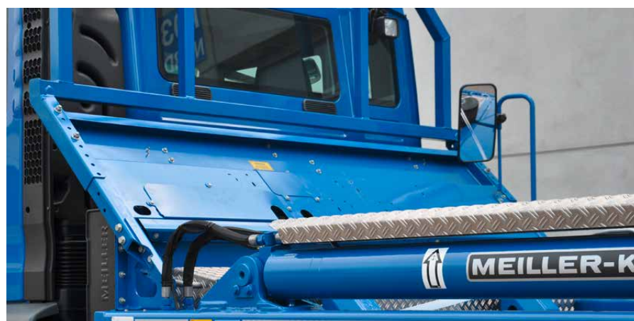
Protection for driver and cab: MEILLER front panel in different versions
