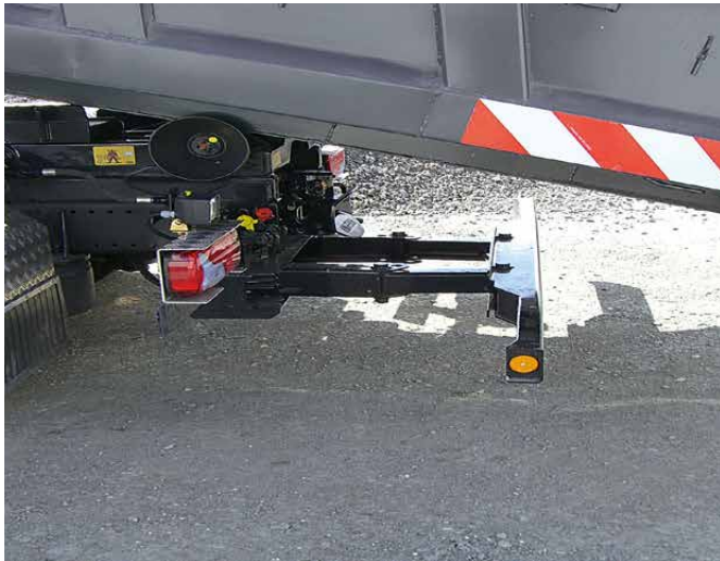
Underride protection extended
