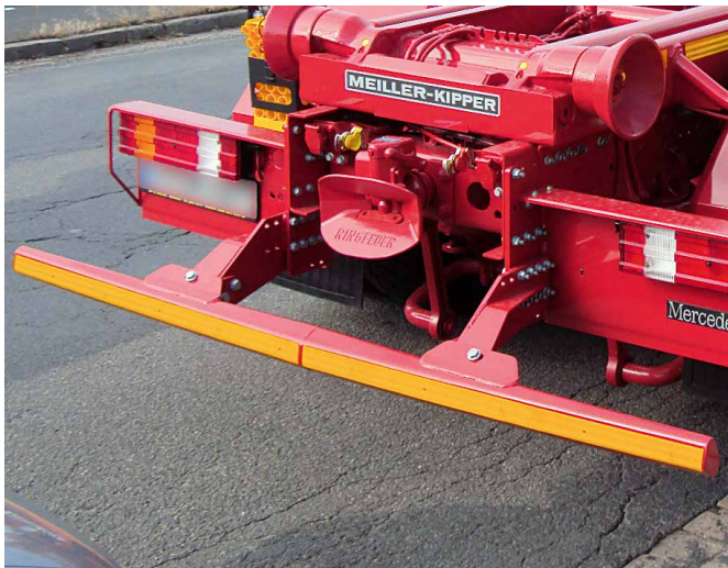
Rigid underride protection
