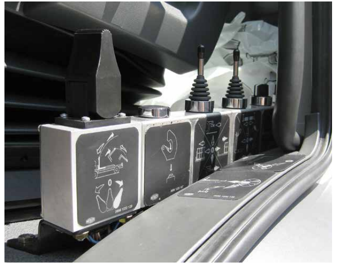
Control units in tilting cab
