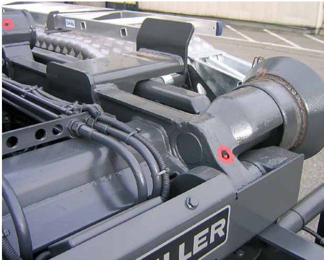
Additional support for short containers
