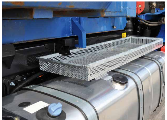
Net box above fuel tank
