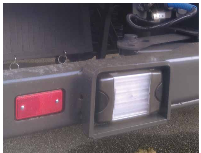
Lighting in the underride protection
