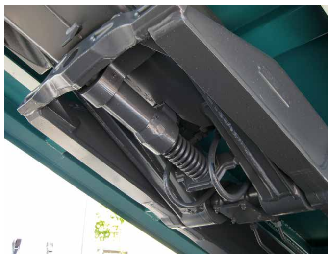
Lifting arm lock
