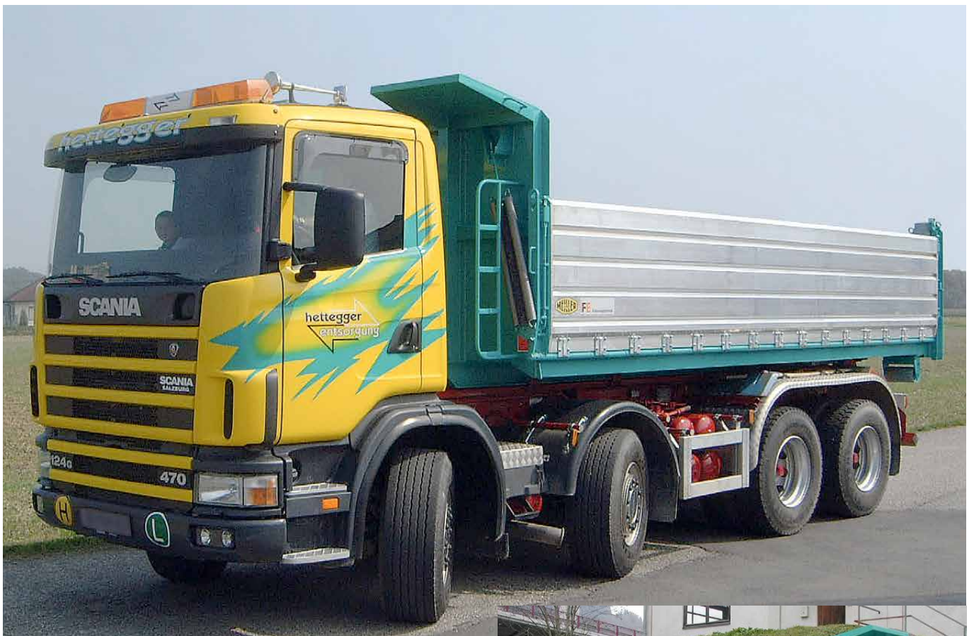
Hooklift with side tipper superstructure
