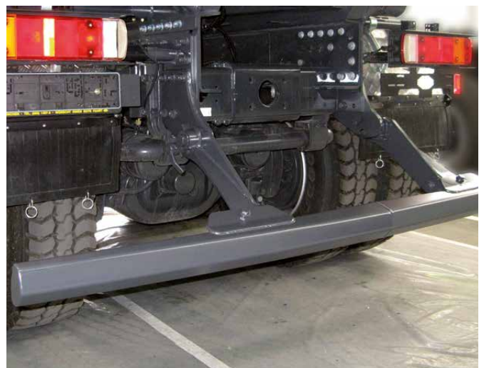
Folding underride protection
