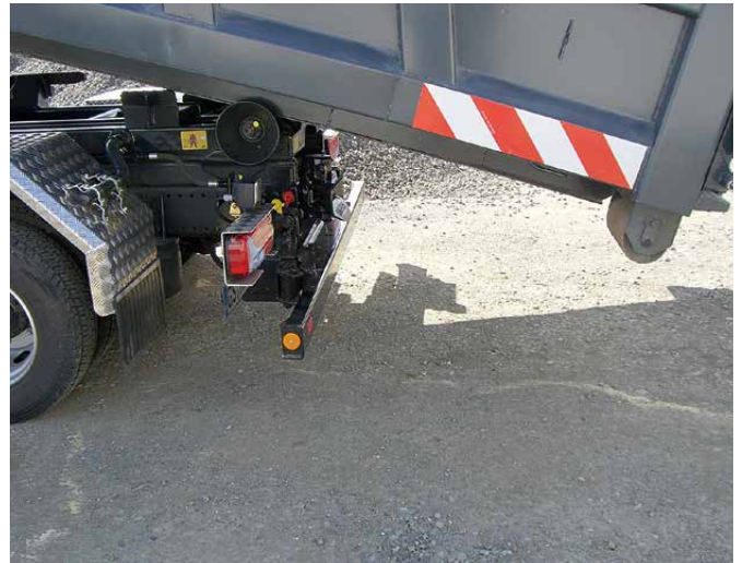
Underride protection retracted
