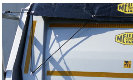
Rear Tipper: Tensioning is easy to handle due to low-lying hooks.
