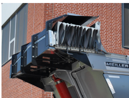
Tipper trailer: Tarpaulin protection roof protects during loading.
