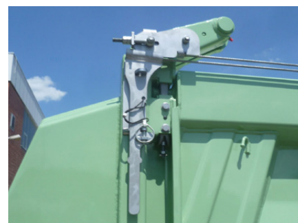
Three-way tipper: Detachable cables due to quick-release fastener.
