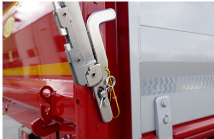
Legally compliant operation: The maximum outer width is adhered to with the flat crank.
