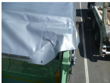
Three-way tipper: Tarpaulin fully covers the tailgate bearing.
