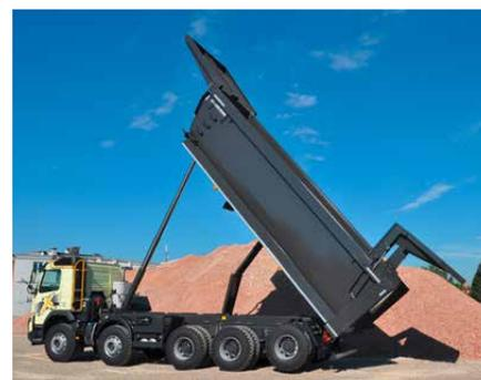
Raised tailgate bearing enables a large throughput e.g. for heavy rubble.
