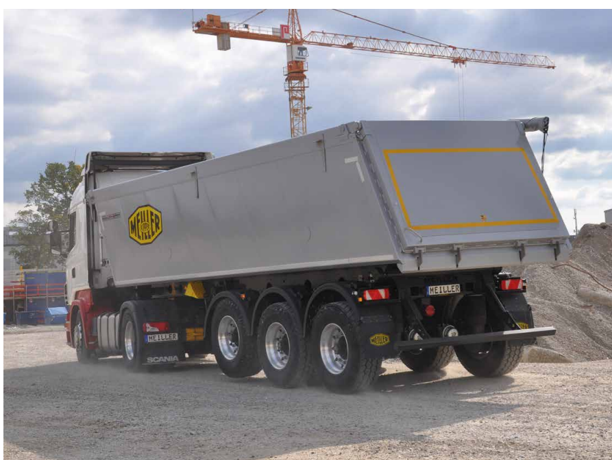
The MHKA tipping semi-trailer with box in aluminium sandwich construction.
