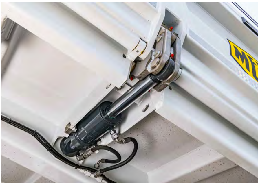
Powerful MEILLER hydraulics at the Bordmatic side wall
