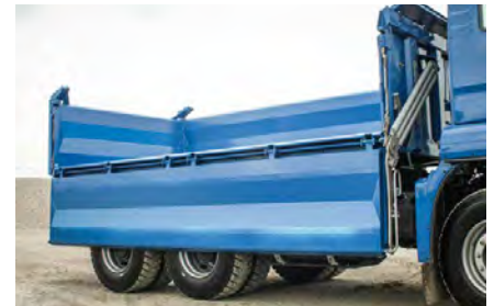
Side wall top-hinged and drop type with relief springs.
