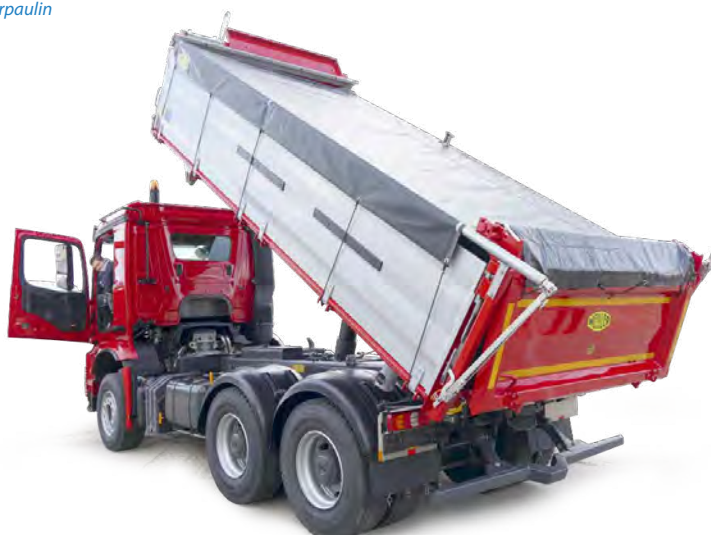
Lateral roll-up tarpaulin operated by crank from the ground
