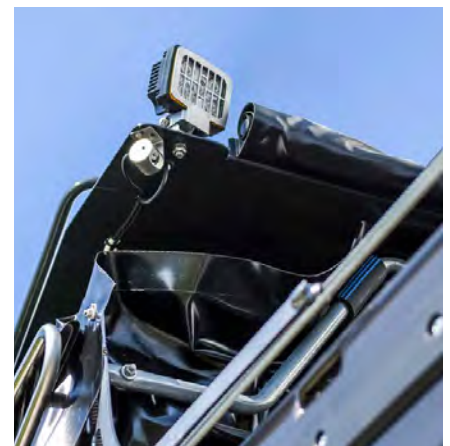
Loading area camera
