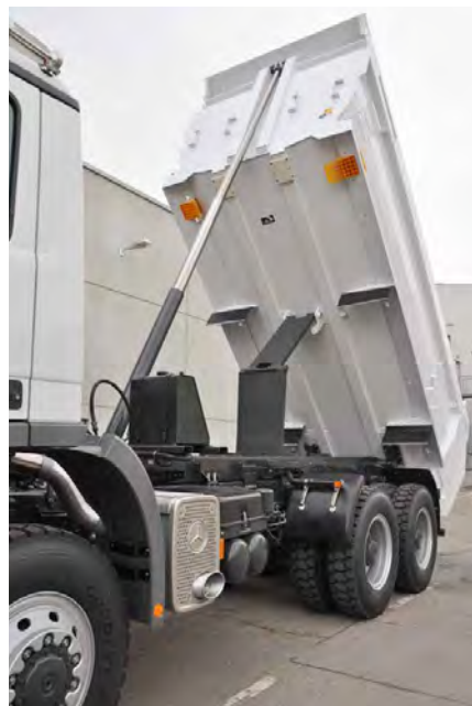
MEILLER scissor tipping stabiliser gives safety when tipping.
