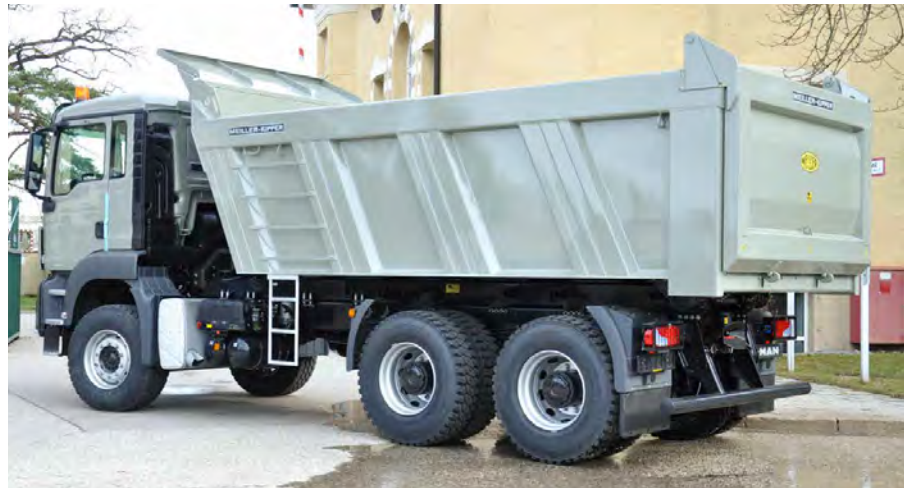
Climb on quickly: Side climb-on with access ladder and treads.
