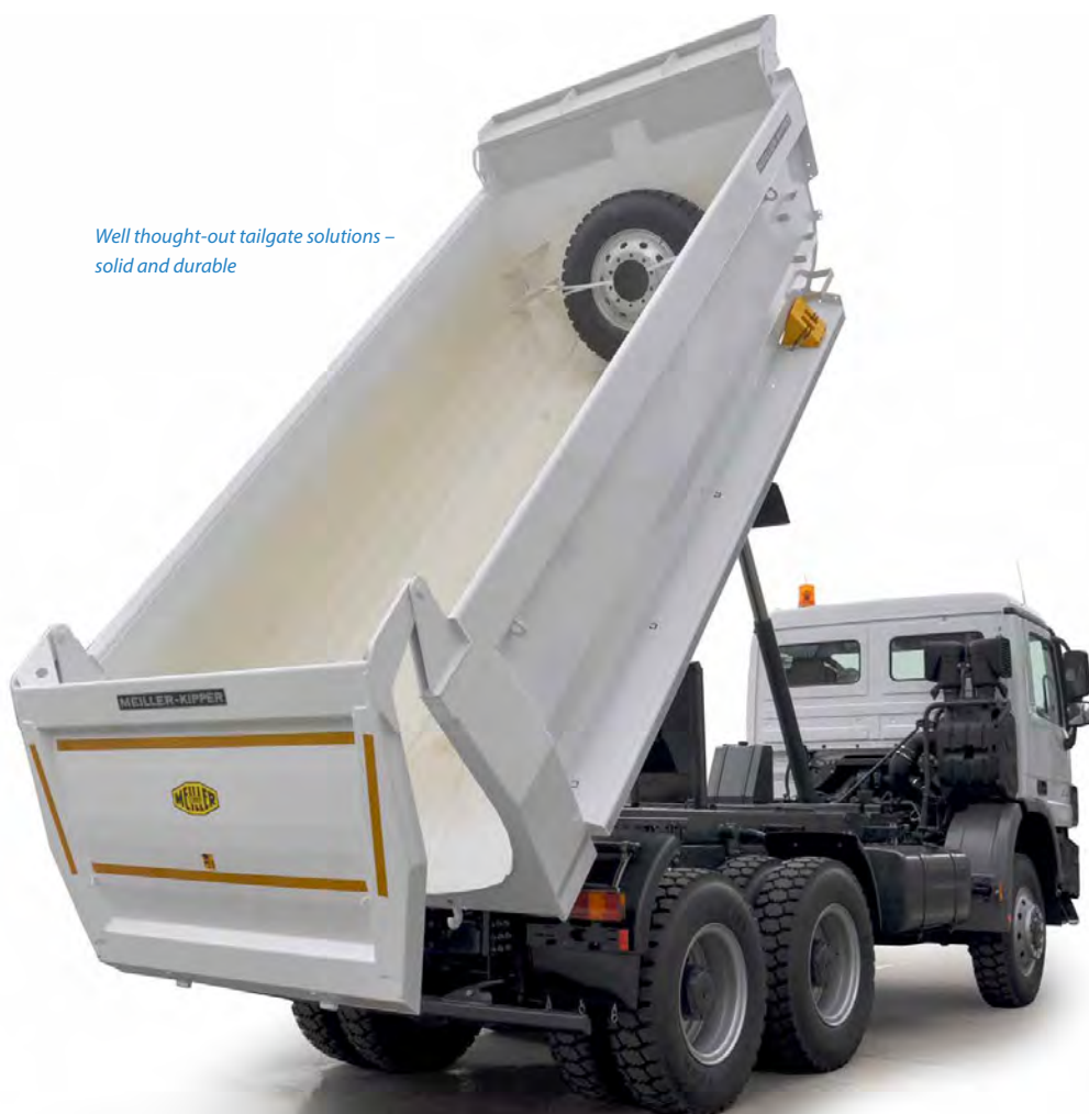
Raised tailgate bearing enables a large throughput e.g. for heavy rubble.
