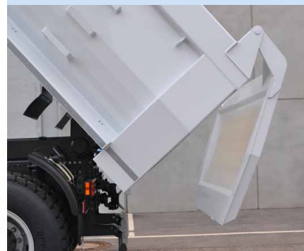
Raised tailgate bearing enables a large throughput e.g. for heavy rubble.
