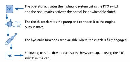
The MEILLER Eco-Kupplung<sup>®</sup> enables you to release power where you really need it. **Engine-driven PTO** MEILLER Eco-Kupplung®
